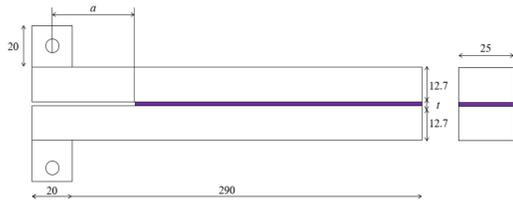
Figure 1 – Specimens' geometry, in mm.
