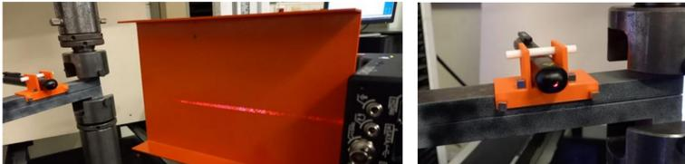
Figure 2 – Laser-based approach for perpendicularity (left) and laser detail (right).
